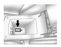
3. Place the new transmitter into the transmitter pocket. The transmitter pocket is inside the center console storage area located between the driver and front passenger seats. The storage area will need to be opened and the storage tray lifted up to access the transmitter pocket.  Press the ignition. When the transmitter is learned the DIC display will show that it is ready to program the next transmitter.
